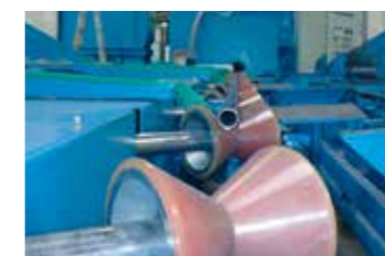
● 处理圆棒，管材的纺锤型辊道通过式抛丸机 Diabolo blast machine for handling sprinkler pipes Diabolo
