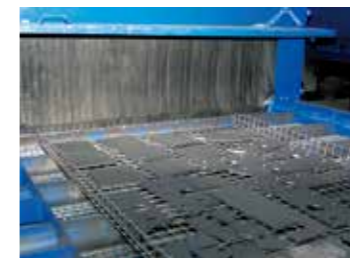
● 带有工件框的切割件通过式抛丸机 Blasting of flame cut pieces in a basket
