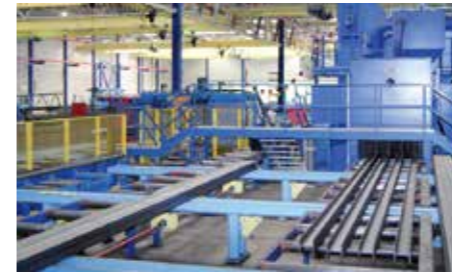
● 带有横移机构的抛丸机 Blast machine with crossover conveyors
