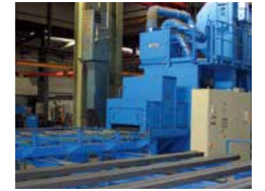
● 带有通过高度可调整的抛丸机 Blast machine with adjustable passage height
