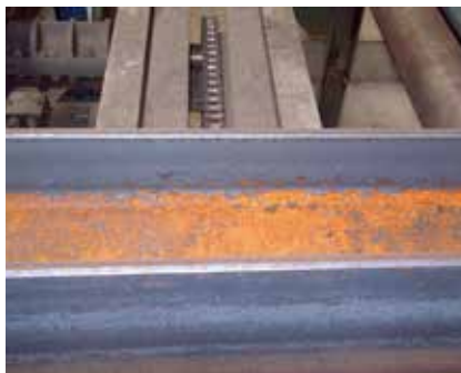
型材抛丸处理之前 Steel beam before...
