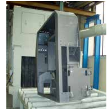
● 用于金属板材，型材及钢结构的抛丸机，其通过高度可达 1000mm Blast machine for metal sheets, sections and constructions with a passage height of up to 1000 mm
