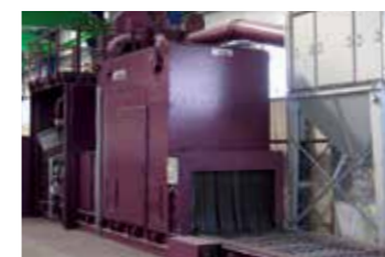
● 用于金属板材，型材及结构件的抛丸机，其通过高度可达 1000mm Blast machine for metal sheets, sections and constructions with a passage height of up to 1000 mm
